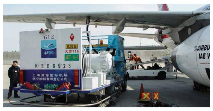
Into-plane refuelling operations at Pudong Airport 浦东机场的飞机加注服务
