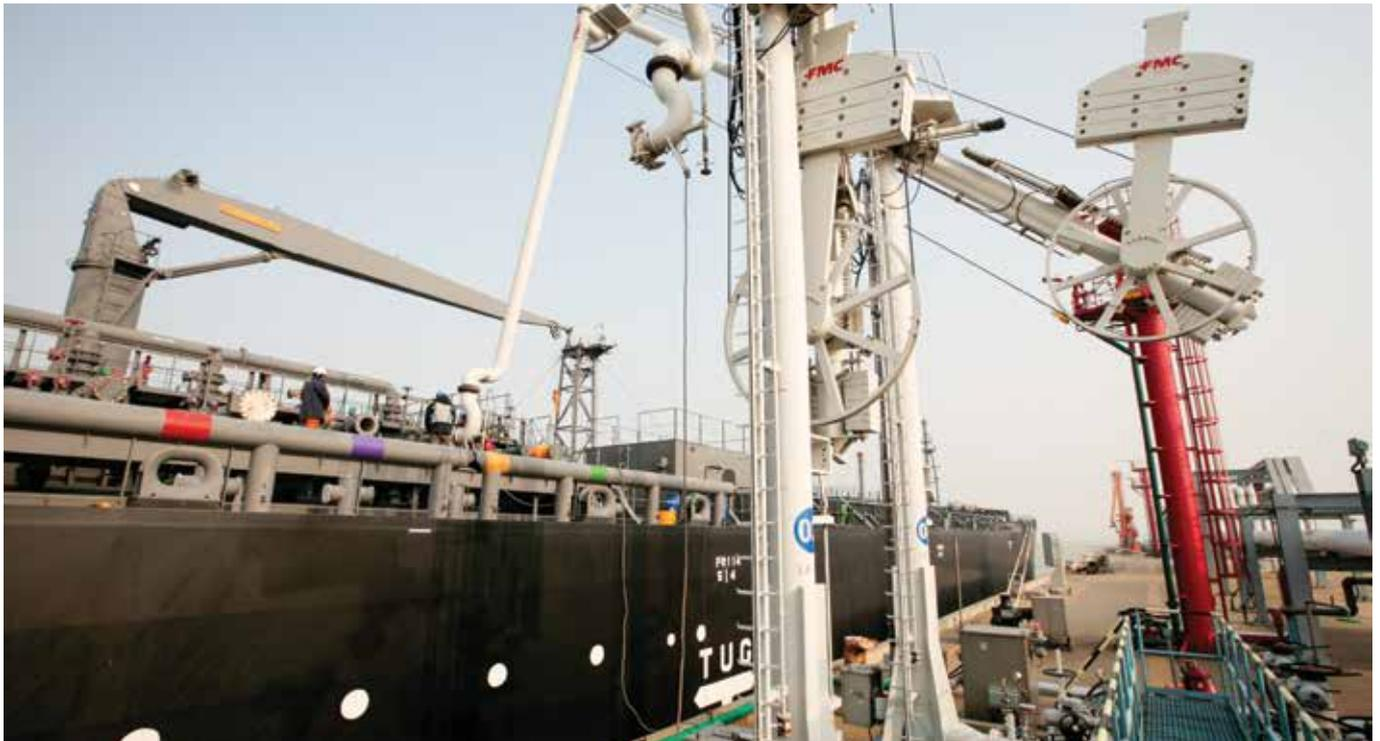
Jet fuel discharging from vessel at port
